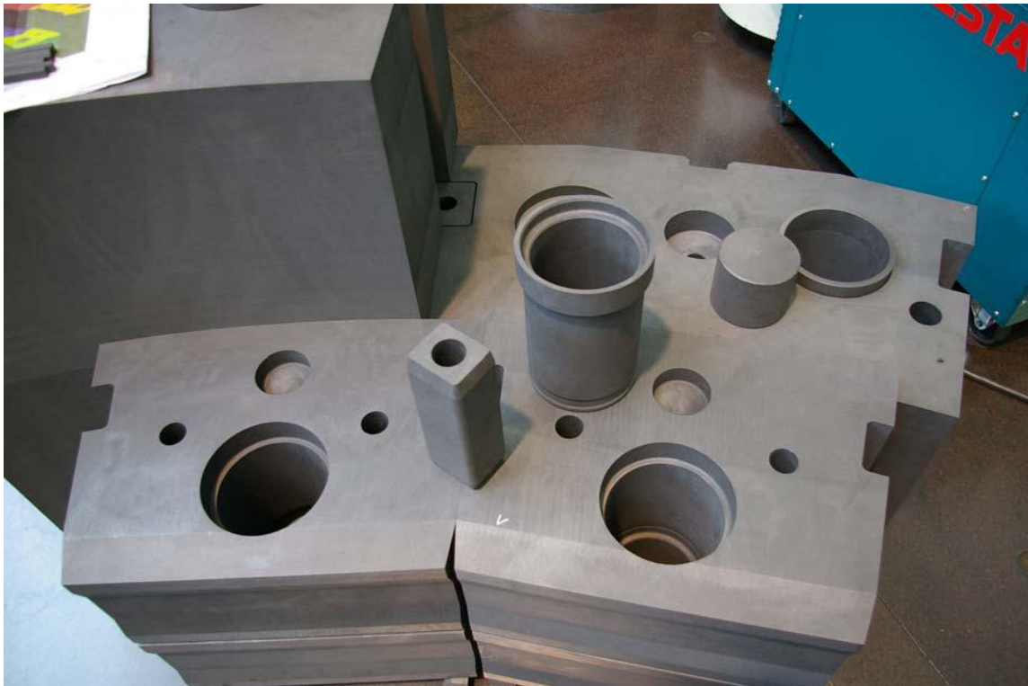
Fig. 6.1: PBMR test assembly of some graphite structural elements
