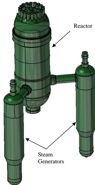
Fig. 2: Nuclear process steam supply system.
