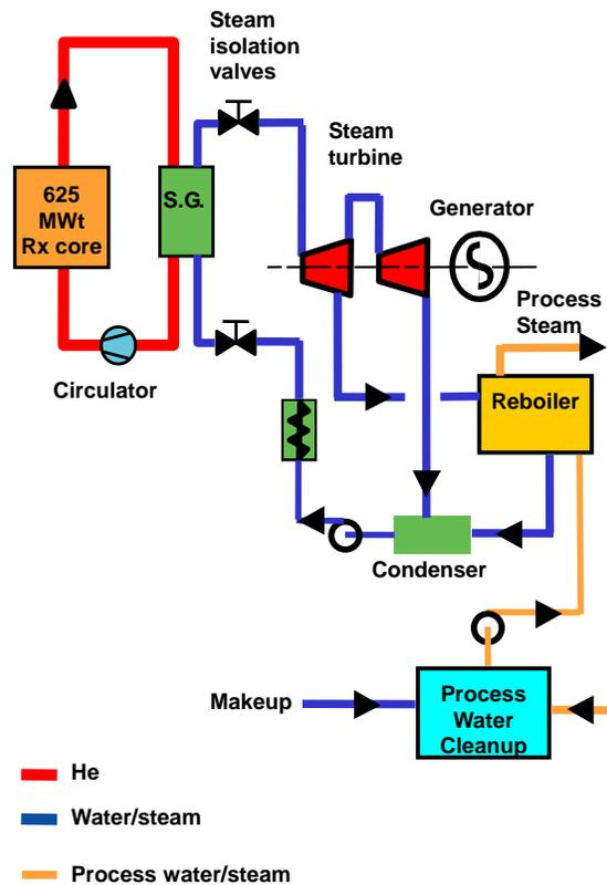
Fig. 5: Typical cogeneration plant configuration.
