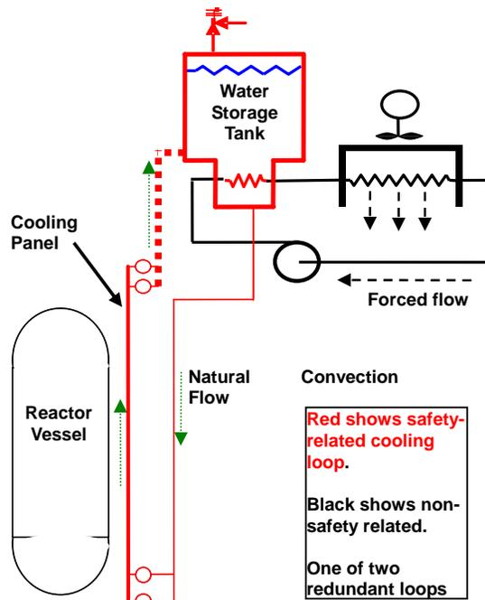
Fig. 4: RCCS schematic.
